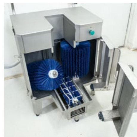
Simple opening for cleaning purposes
